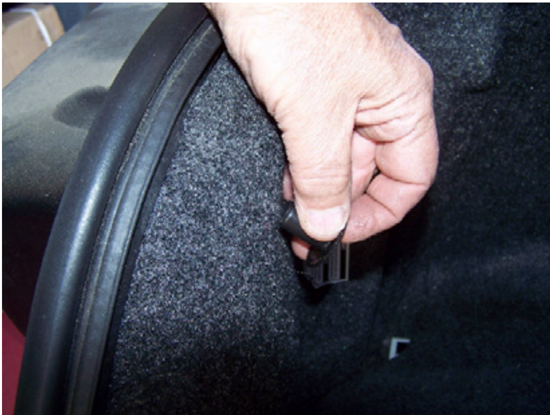
Unscrew and remove threaded plastic barrel fitting
