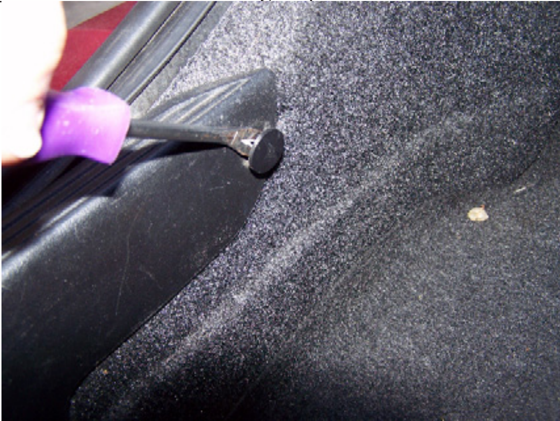
Locate and pry out plastic serrated lower trunk trim retainer
